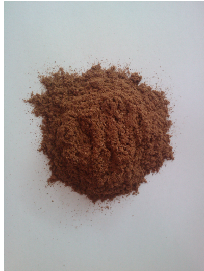
Figure 18 WF treated for 60 min at 220 °C
