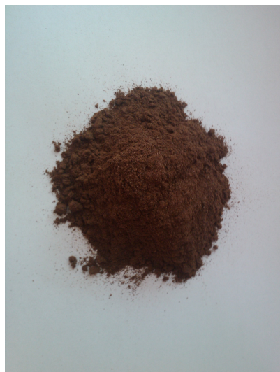
Figure 22 WF treated for 5 min at 260 °C
