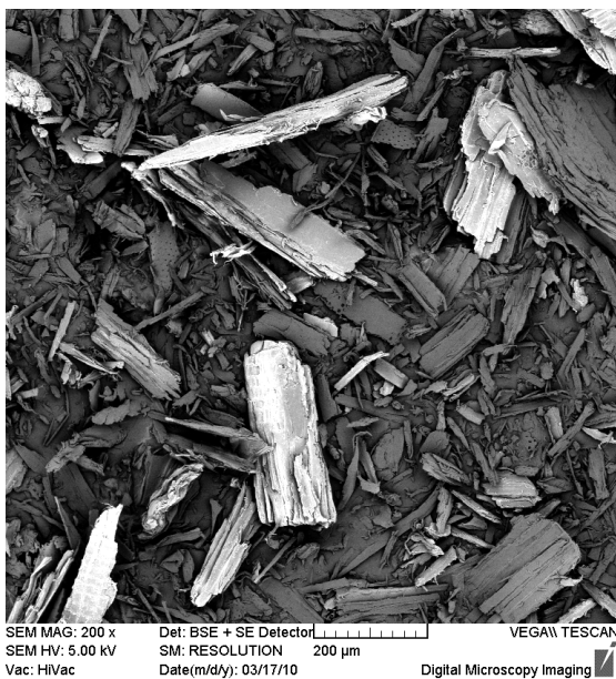
Figure 12 SEM micrograph of WF retified for 5 min at 260 °C
