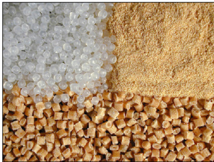
Figure 1 WPC – top left: polyethylene granules, top right: wood flour, bottom: wood-plastic composite pellets [11]
