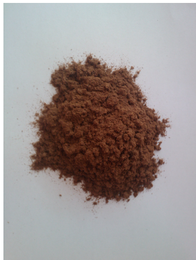
Figure 20 WF treated for 5 min at 240 °C
