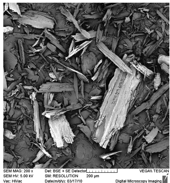
Figure 9 SEM micrograph of WF retified for 5 min at 220 °C
