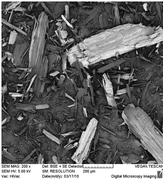
Figure 10 SEM micrograph of WF retified for 60 min at 220 °C
