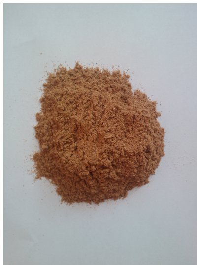
Figure 16 WF treated for 5 min at 220 °C
