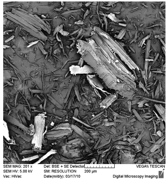
Figure 11 SEM micrograph of WF retified for 5 min at 240 °C
