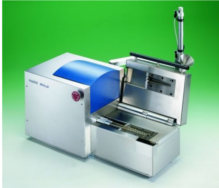
Figure 13 Haake Minilab Rheomex microcompounder intermeshing co-rotating twin screw extruder
