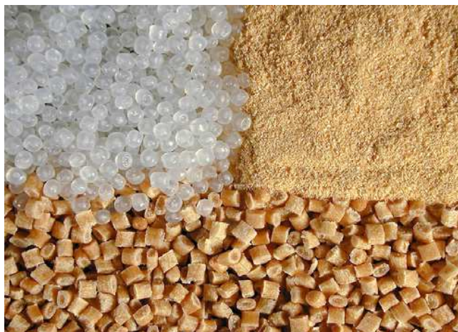
Fig. 3. Compounded pellets (bottom) made from wood (upper right) and plastic (upper left).
