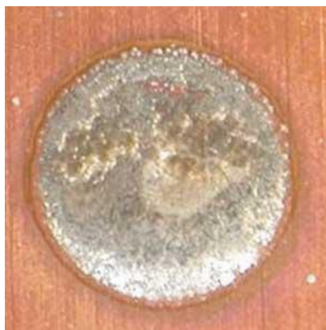
Obr. 33 Porucha Poor Wetting
