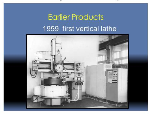
"The company had passed through several development periods of machinery manufacturing. In 1959 the company manufactured the first vertical lathe with continuous feeds and with the NC line motion control system equipped with the copying attachment. This vertical lathe was made on the basis of the company's own documentation. The really interesting thing is that the plant started manufacturing this generation of machines as one of the first ones in the world."
