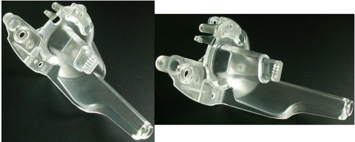
Figure 38 Cavity side of the LED holder
