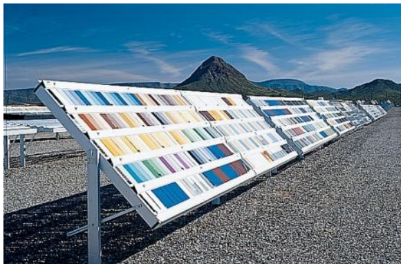
Figure 8 - Weathering site in Arizona, USA [38]
