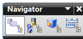
Obr. 36. Program Order View, Machine Tool View, Geometry View a Machining Method View
