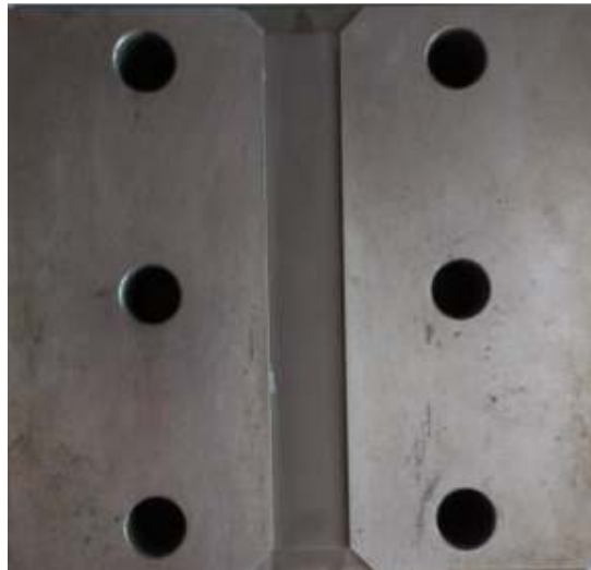
Fig. 16. Representation of slit die geometry with parameters (15/1/100) mm and roughened surface
