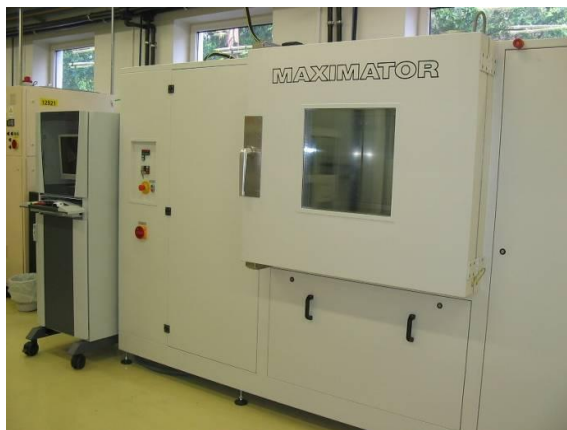
Figure 29: Test stand Maximator with mass spectrometer INOVA 1314
