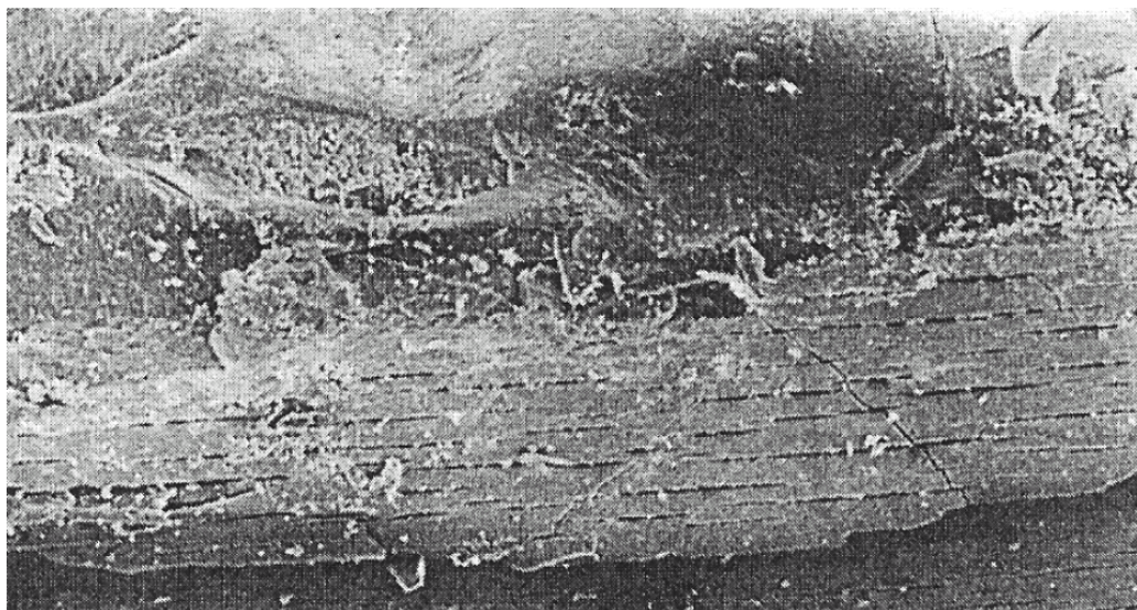
Fig. 7. Cracks in the surface of polypropylene samples during tensile testing after 12 weeks laboratory UV exposure while held in bending [58]
