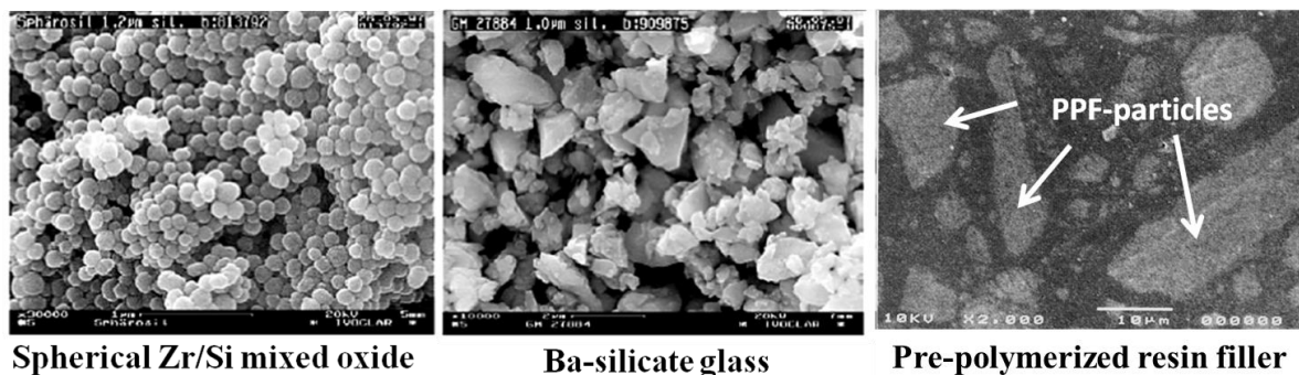
Fig. 5 SEM pictures of different fillers with different sizes and shapes used in VLC RBCs [21,51].
