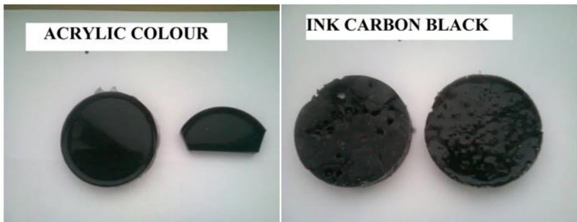
Figure 25- Examples of different pigments mixed with SR
