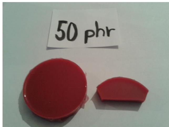
Figure 26- Calibration object with 50 phr of GS and pigmented by red tempera
