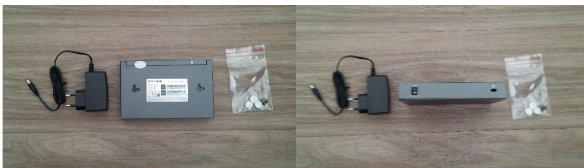
Obr. 13. L2 switch TP-LINK TL-SG108E.
