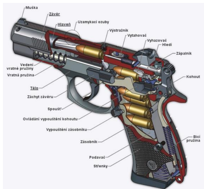
Obr. 6. Detail mechanismu pistole [3]
