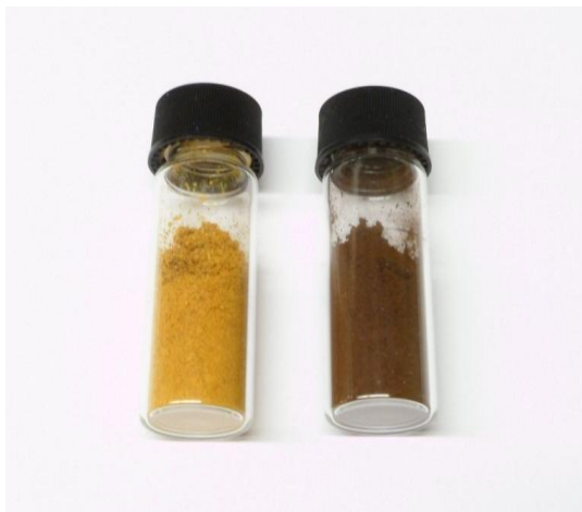
Figure 29: difference in colour between Poly(DEB) and Poly(DET)
