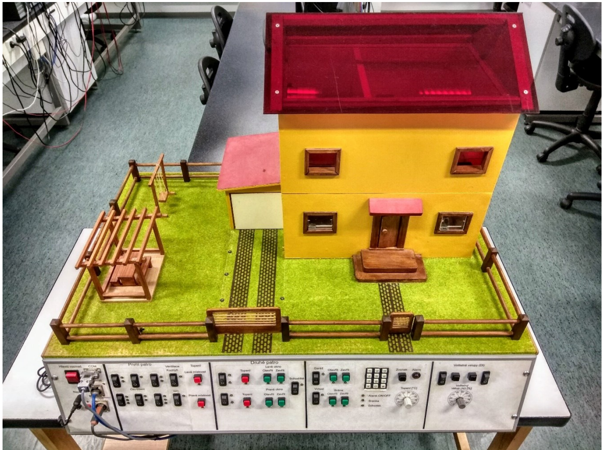
Figure 5: 1:30 model of a house connected to a Saia PCD2
