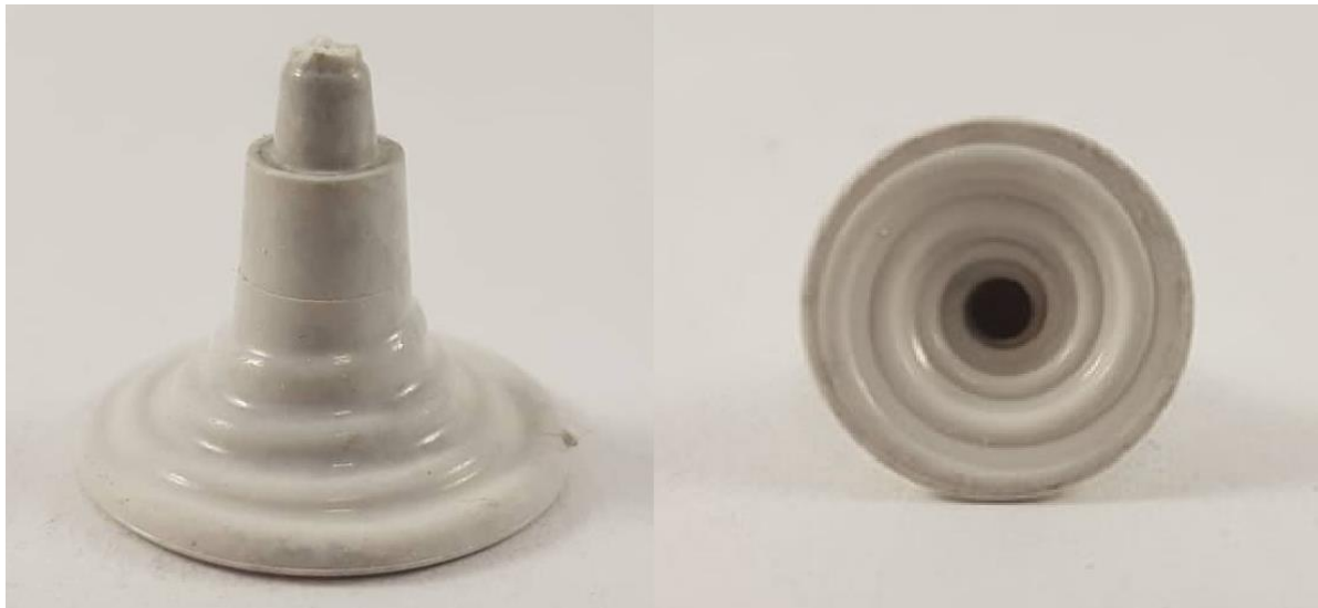
Figure 16 – Design of tested Al_2O_3 PIM part
