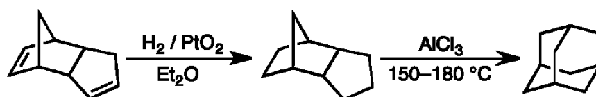
Scheme 1: Schleyer's synthesis of adamantane.
