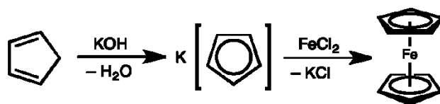
Scheme 3: Synthesis of ferrocene published by Pauson and Kealy.
