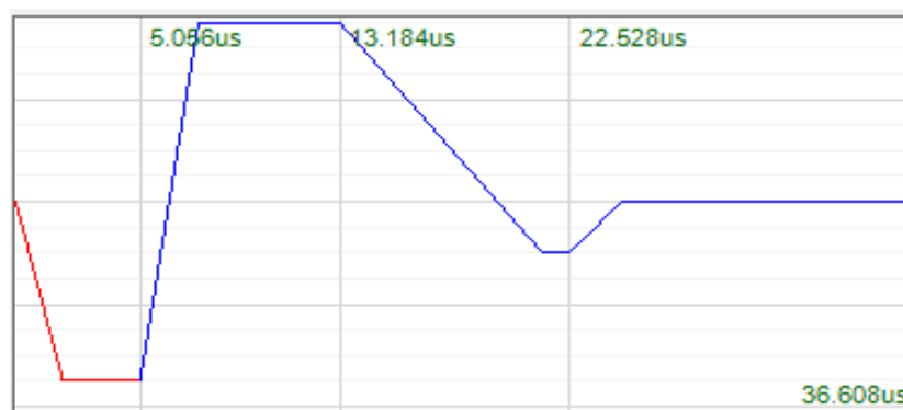
Figure 25 An example of a waveform which was used for printing of CuO layers.
