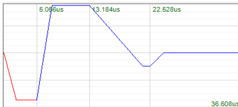
Figure 11 An example of a waveform which was used for the printing of CuO layers. [own source]
