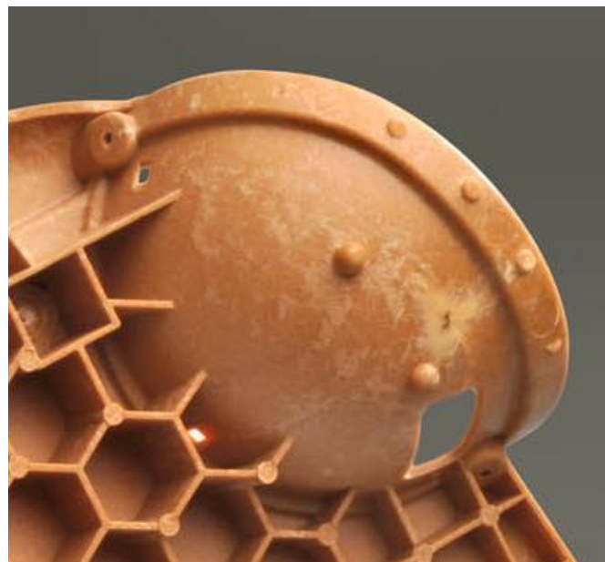
Fig. 27 - Phase separation on highly highly filledfilled WPC compound (Duretek, 2016)
