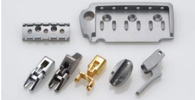
Fig. 4 - Examples of consumer products made by PIM (Otsuka 2018)
