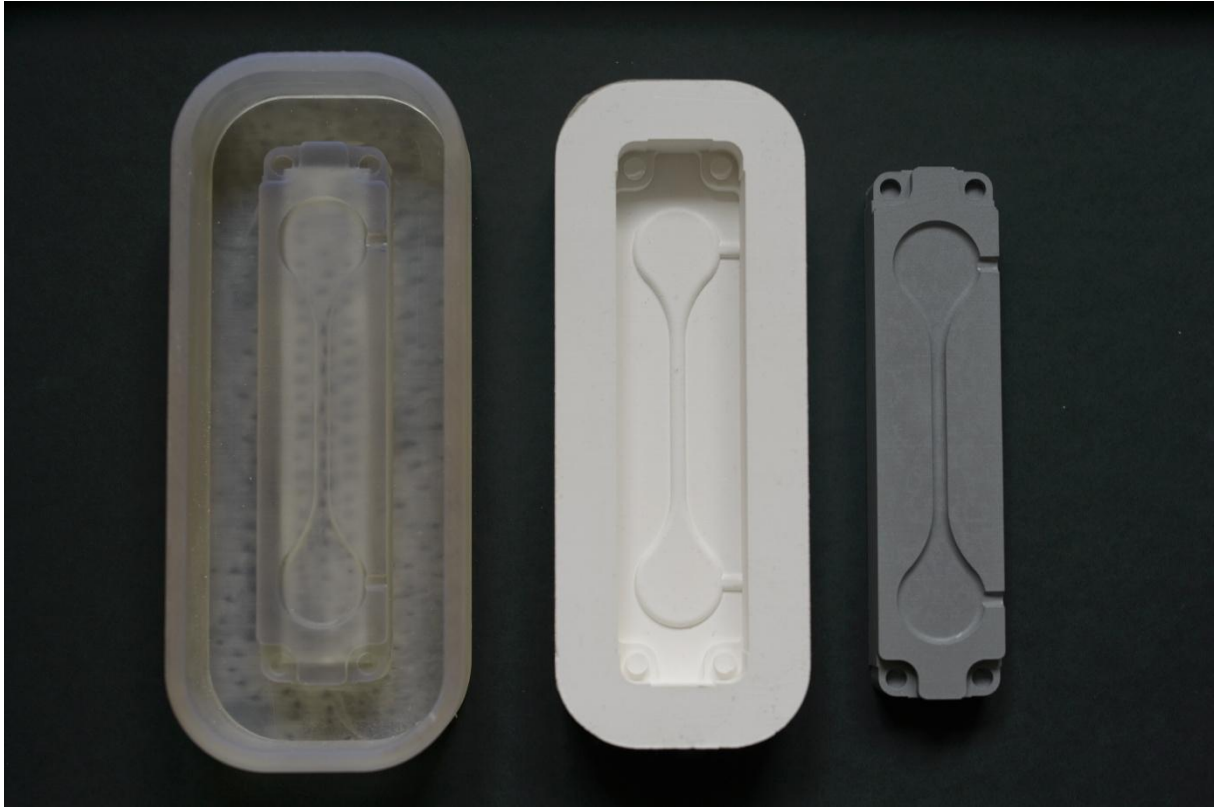
Fig. 61 - 3D printed model (left), negative silicon mold (middle), final insert from epoxy resin (right)
