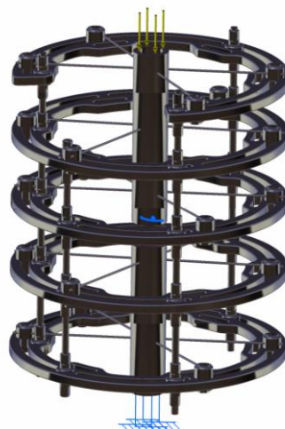
Fig. 5.2: External fixator loading during all the deformation tests
