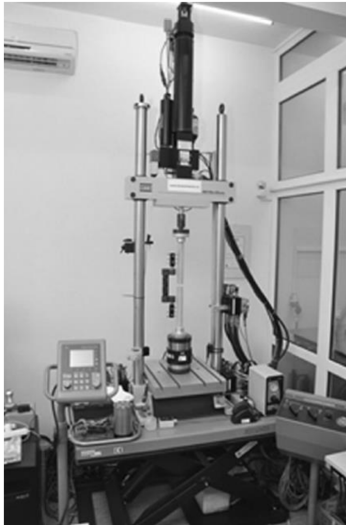
Fig. 3.7: The testing system for external fixator loading
