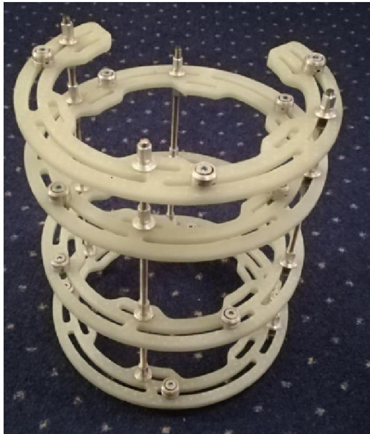
Fig. 5.12: Assembled external fixator with composite rings
