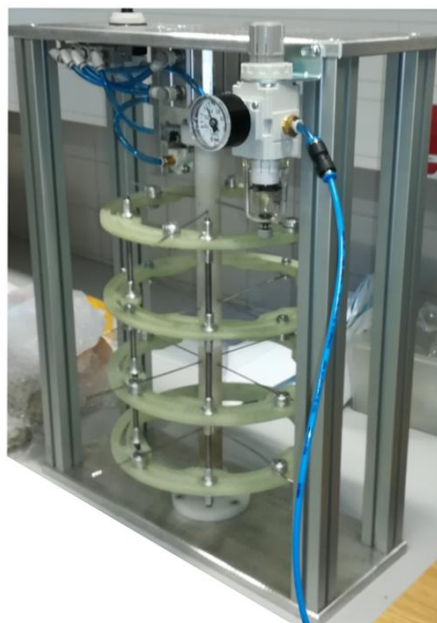
Fig. 5.15: Cyclic testing machine manufactured by Matěj Homola connected with the manufactured external fixator
