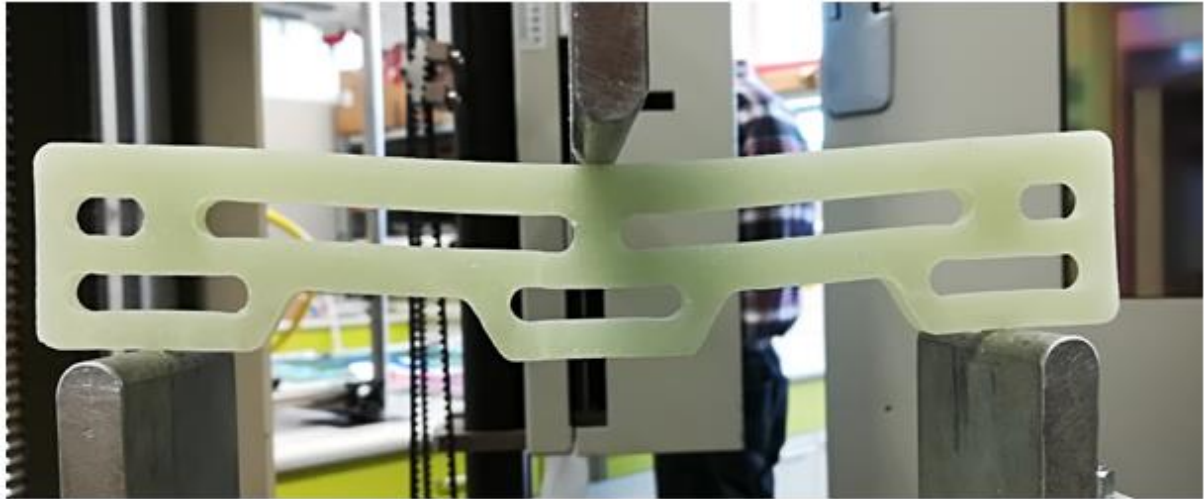
Fig. 5.8: Loading of the specimen by the three-point bending in the first direction
