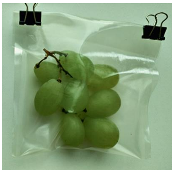
Figure 3: The food package prepared with “PVP-CMC” hydrogel film 20
