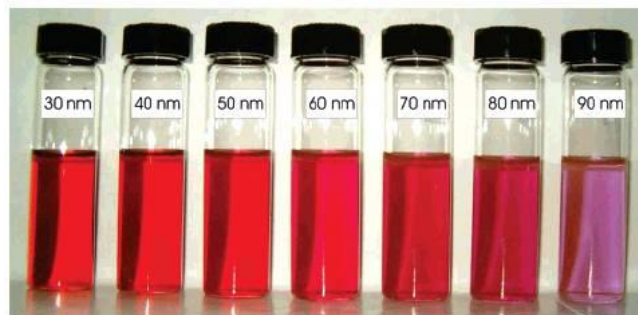
Fig. 1.1 Colloidal Au nanoparticle with different particle sizes [1].
