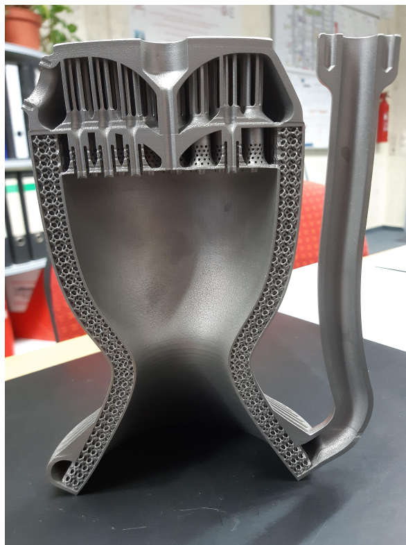
Figure 1.4 3D printed SuperDraco rocket engine core [11]
