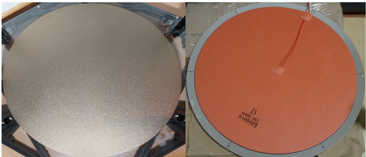
Figure 8.6 Bed - assembly top side (left) bottom side (right)
