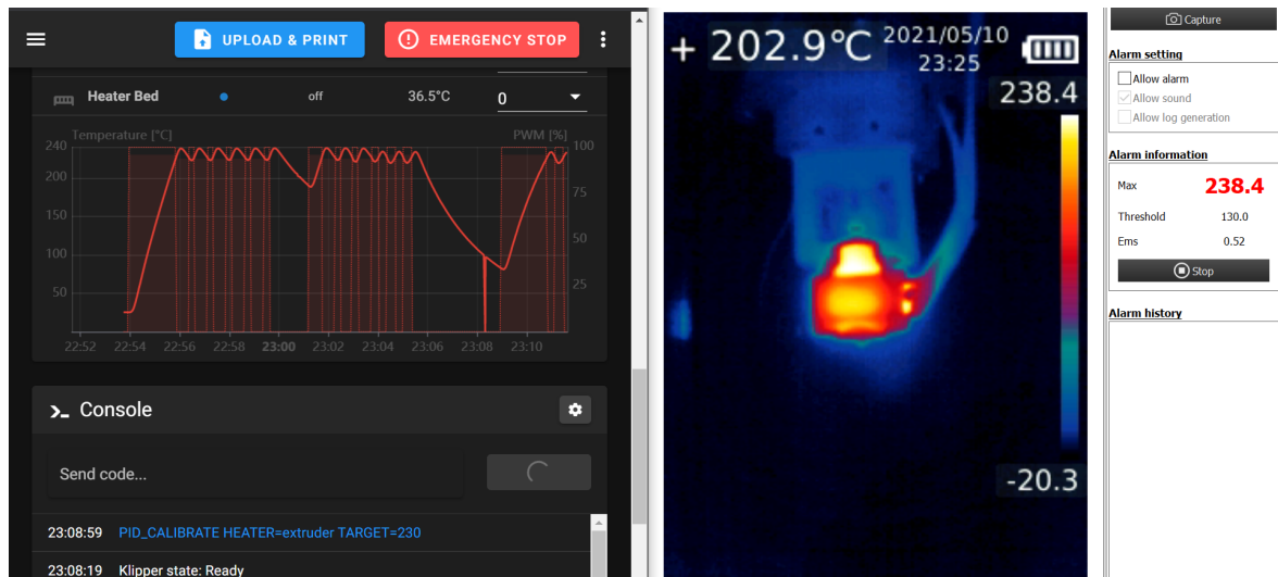
Figure 9.4 Hot-end temperature graph and thermal view from UNI-T 260B
