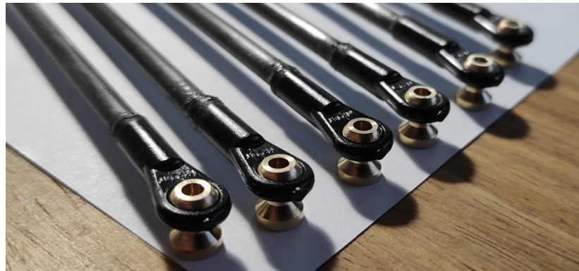
Figure 7.14 Carbon rods with MP-Jet V2 joints
