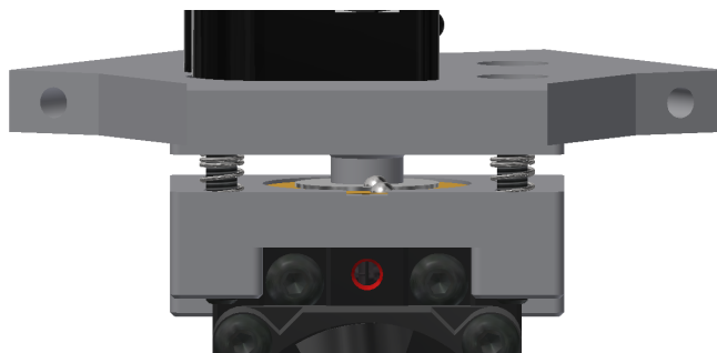
Figure 7.19 Effector with a piezo levelling sensor
