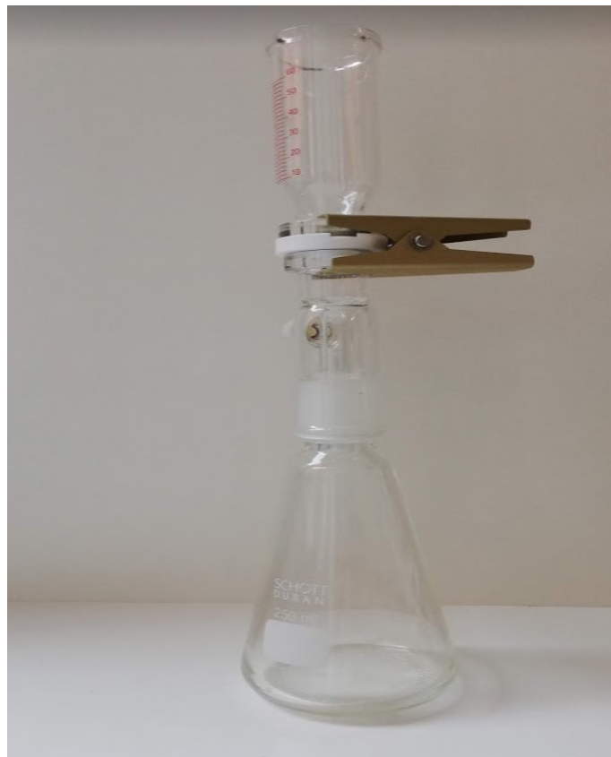
Picture 4 Vacuum filtration equipment for measuring the rate of liquid leakage of the sample
