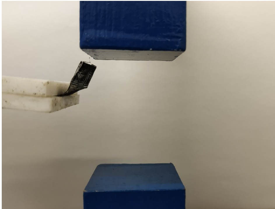
Figure 69 Image of the scaffold 50% in the presence of magnetic field strength, 80 kA/m.
