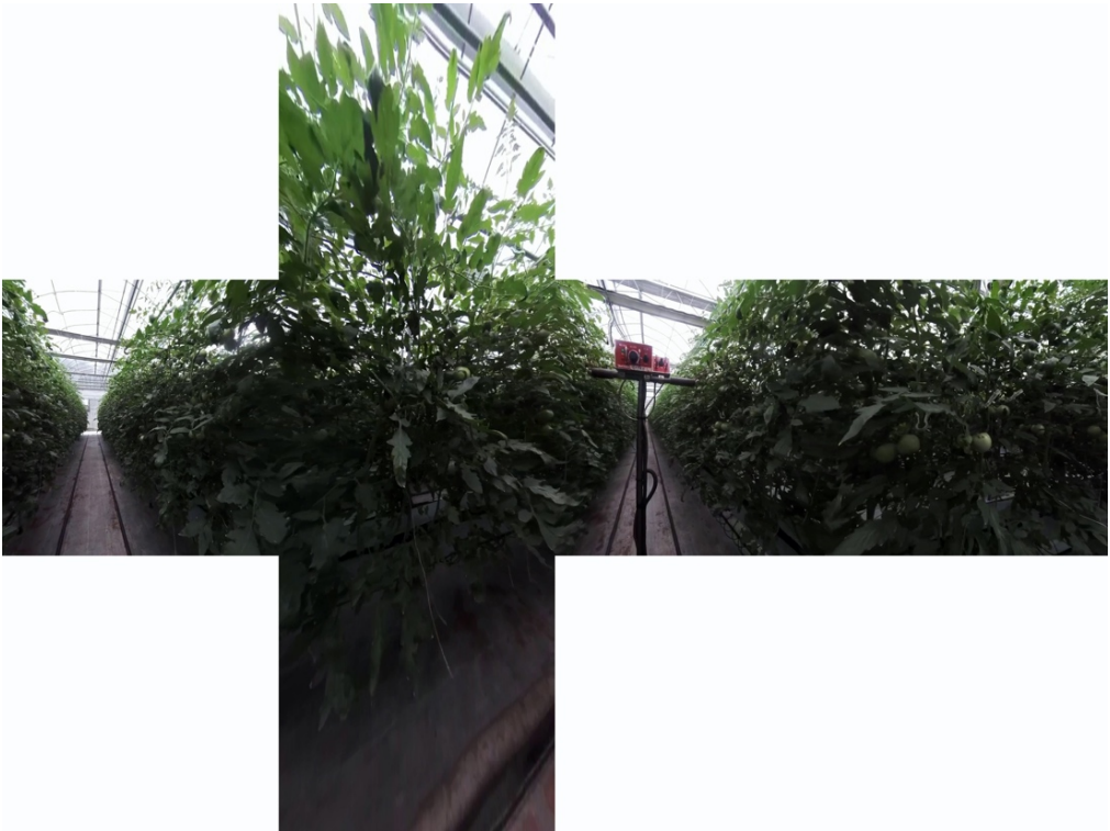
Fig. 5.2 Projection of a 360-degree camera frame into two planes, only the vertical part is utilized in the final image reconstruction.
