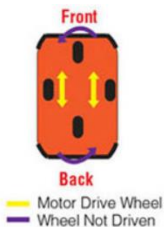
Obrázek 10 Differential drive (Orientalmotor, ©2022)
