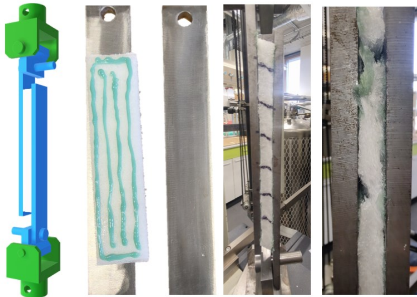
Figure 28 – From left: 3D model of testing apparatus, pattern for application of adhesive, shear test with visible inhomogeneities in samples, end of shear test with visible deformations.
