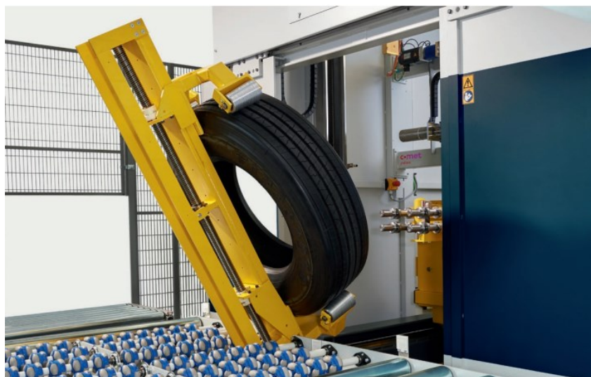
Figure 23 Tire manipulator for loading tires into MTIS system from conveying system [1]
