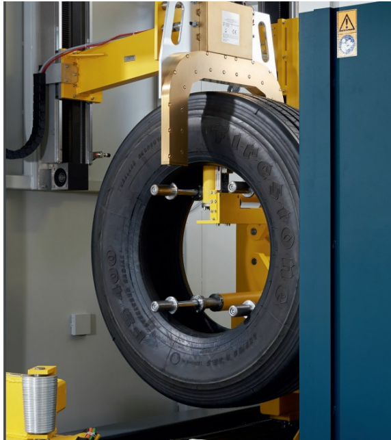
Figure 24 UScan3 line detector and 4-spindle tire manipulator [1]
