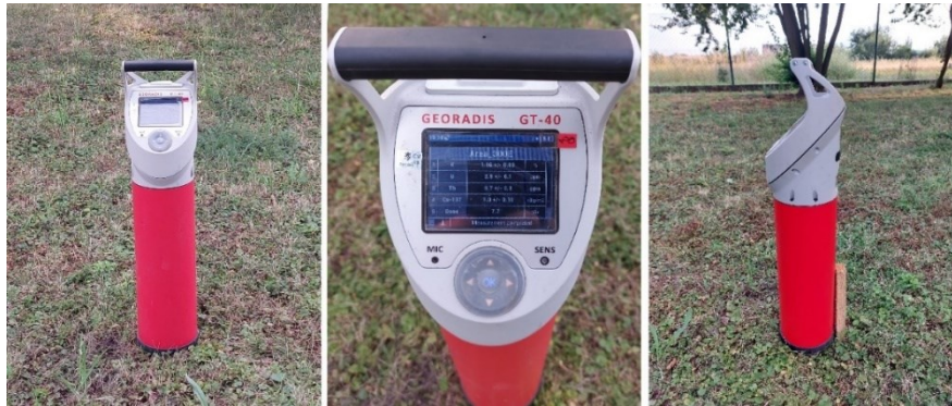
Figure 48. GT 40 – multipurpose portable gamma spectrometer.
