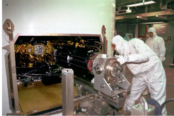
Figure 25. Installation of one of three radioisotope thermoelectric generators (RTG) on the Cassini spacecraft (Plutonium ^{238}\text{Pu} ) [58].
