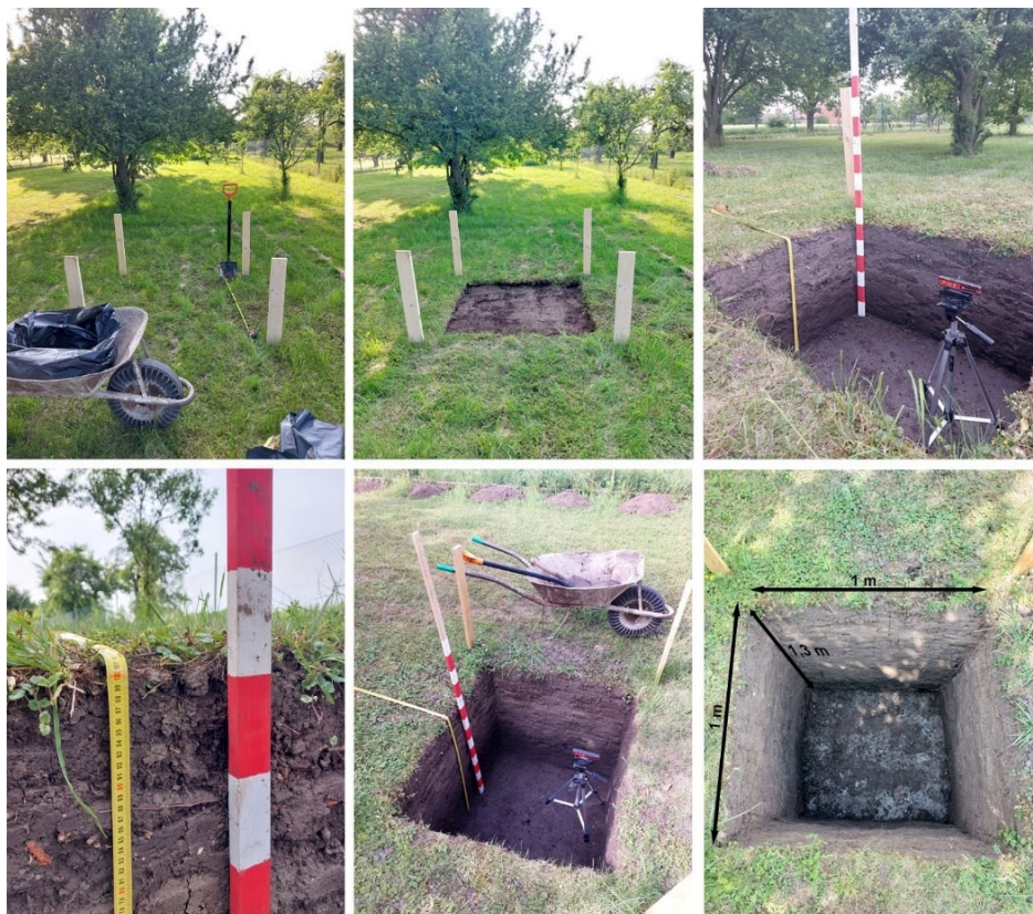
Figure 73. The procedure and measurement of the sampling of each layer.
