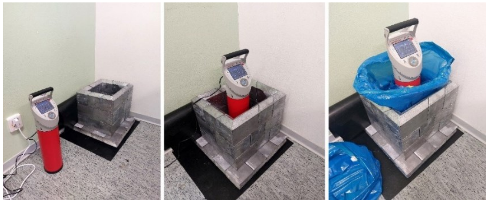
Figure 86. Measurement of individual layers in the lead box.
