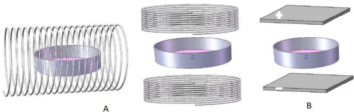
Figure 5 (A) Cell culture placed inside one Helmholtz coil, or place between two Helmholtz coils; (B) Cell culture placed between two parallel plates (Meng et al., 2022)
