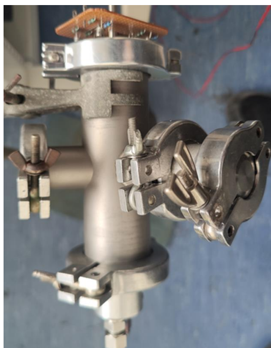
Figure 5.1: Schematic of the gas sensing system (above) and the sensing chamber with the sensor holder with the chamber lid (below).
