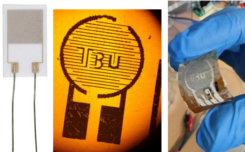
Figure 4.2:(a) Schematic of prefabricated sensor and interdigit motif for sensor (above) (b) coated ceramic and flexible inkjet printed sensor before and after growth (below)
