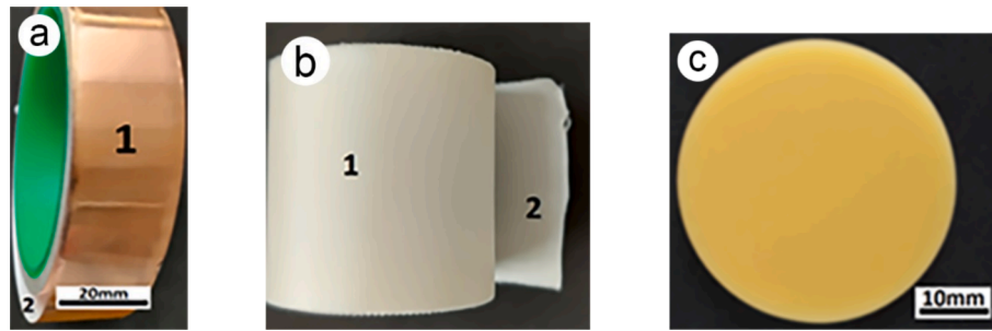
Fig. 5. (a) Copper foil (pos. 1). Paper band on the side with electroconductive adhesive. (b) Surgical tape roll (pos. 1). The adhesive side of the tape (pos. 2). (c) Natural rubber pad.
