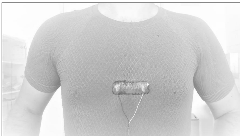
Figure 7. Sensor based of MWCNT (KMnO 4 ) fixed on a sports T-shirt for practical application of a human breath monitoring.
