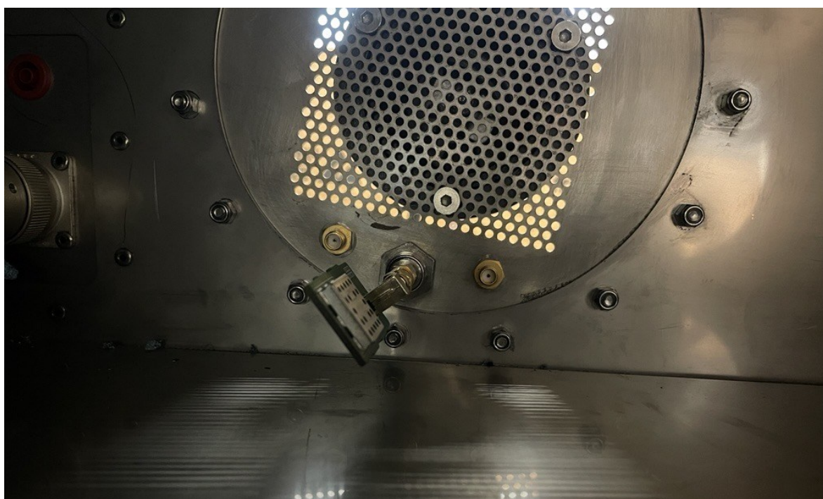
Figure 21 Measurement in GTEM cell with BLS. [Own]
