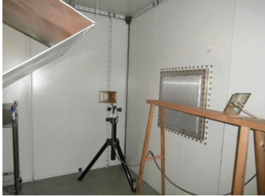
Figure 5 Stirred Reverberation chambre. [14]
