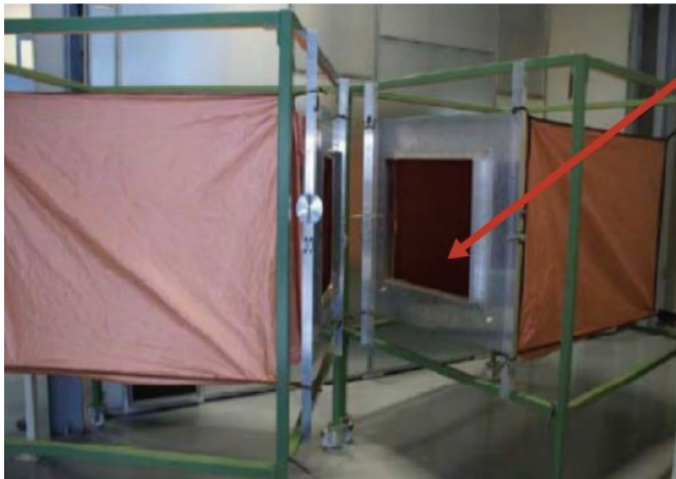
Figure 8 Two VIRC chambers made of flexible material, with a red mark indicating the sample location.[14]
