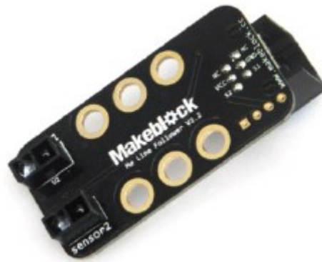
Figure 14 Me Line Follower v1.2 sensor detects lines using dual infrared reflectance for navigation
