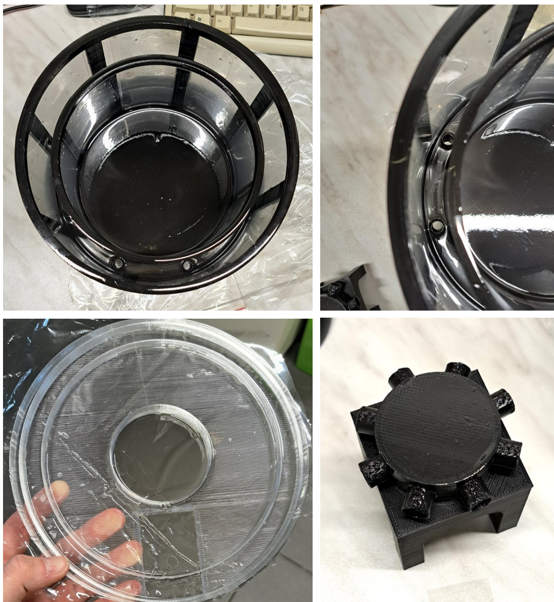
Figure 72 – Photographs of the custom atmospheric chamber during construction.
