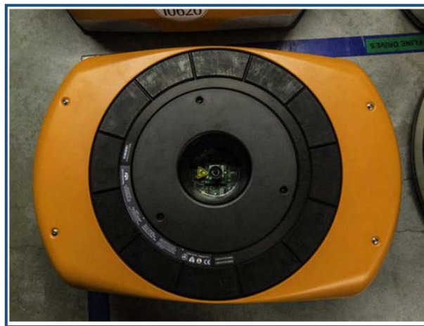
Figure 8 Kiva robots equipped with cameras (Source: Li and Liu, 2016)
