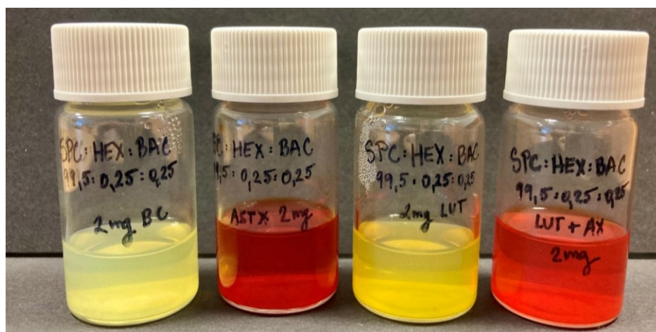
Figure 43: Final SPC:HEX:BAC formulations with encapsulated (from the left) \beta -carotene astaxanthin, lutein and mixture of astaxanthin/lutein, 2 weeks after preparation
