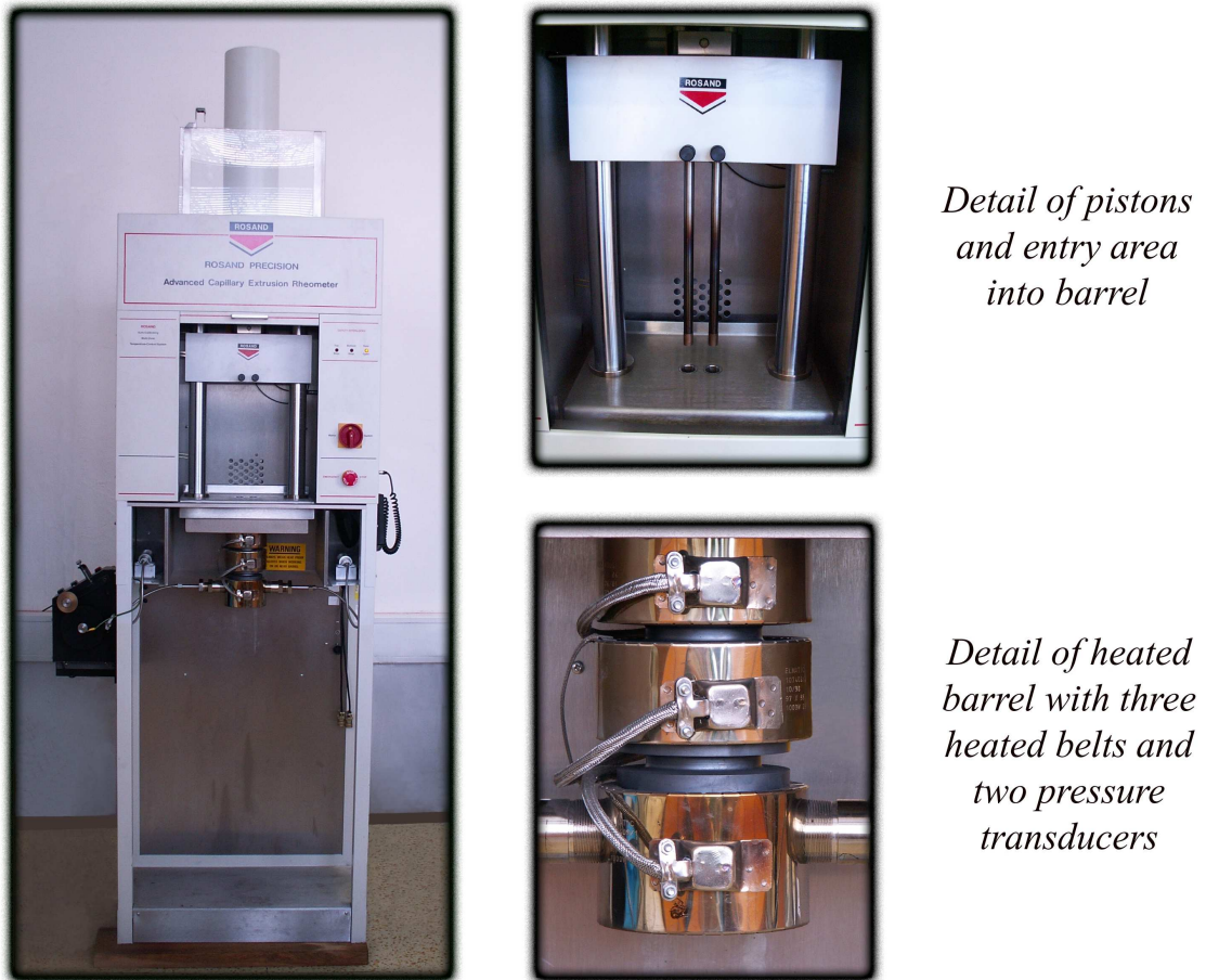
Fig. 40: Real view of twin-bore capillary rheometer ROSAND RH7-2
