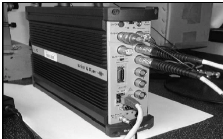
Fig. 15: Three-channel portable PULSE multi-analyzer Brüel&Kjaer, type 3560-B-030 [45].
