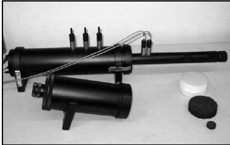
Fig. 16: Two-microphone impedance tube Brüel&Kjaer [45].
