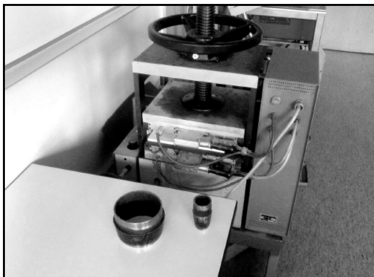
Fig. 19: Cold press and cutting knives for sample preparation [46].
